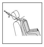
If the position you are using has an adjustable headrest or head restraint and you are using a single tether, route the tether under the headrest or head restraint and in between the headrest or head restraint posts.
